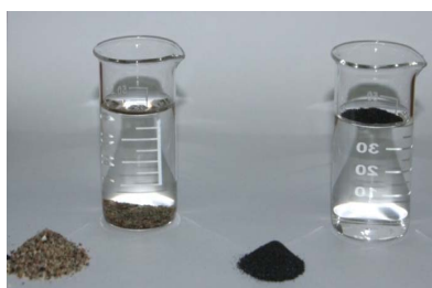
Fig. 1. Properties of hydrophobic sand: 1 – usual river sand on the bottom of glass; 2 – hydrophobic sand on the surface of water.
